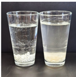
◀ Comparison of action in water after 12 hours: on the left, the medium used in KalyxX 100 mini, on the right, polyphosphates.
